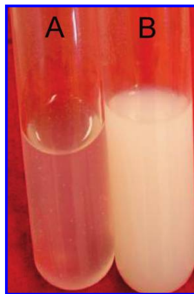
Figure 4. Paste clarity from a typical cassava starch (A) and from the small-granule mutation (B).
